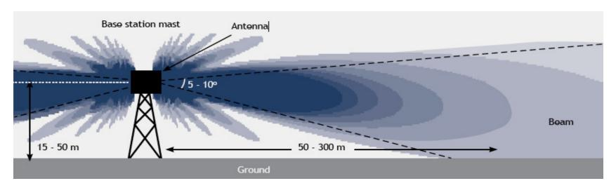
Propagation of "main beam" from antenna mounted on a tower or roof top
