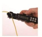
**VISUAL FAULT LOCATOR / FIBER PATCH CORD**
